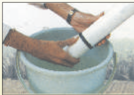
Don't use oil on threads of X-illant column pipes and always clean the thread of pipes with water before use and check the proper fitment of rubber sealing element.
